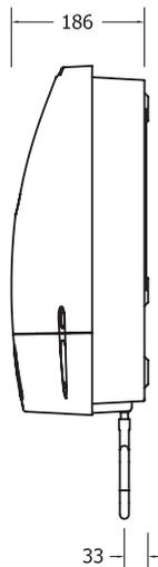
**Model:** GP-DMI-STD-2 - Mechline's GreasePak, battery operated, biological drain maintenance system.
