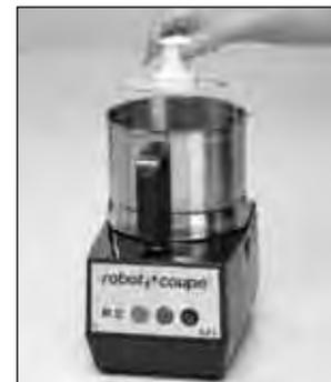
3) Engage the blade on the motor shaft and lower it right to the bottom of the bowl.
